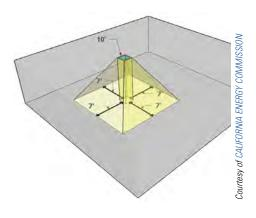
The **skylit daylit zone** is an area of the space equal to the area of the skylight plus a distance 0.7 times the average height of the skylight above the floor, extending out from the edges of the skylight
