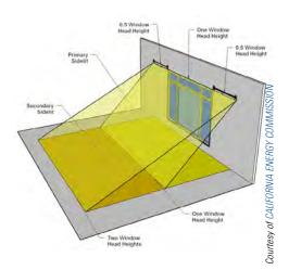
The primary sidelit daylit zone is an area on a plan directly adjacent to each vertical glazing, one window head height deep into the area, and window width plus 0.5 times window head height wide on each side of the rough opening of the window.
